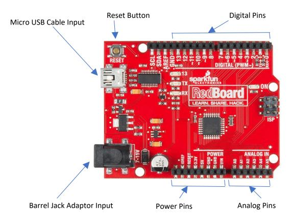
Reset Button: Used when restarting the code programmed on the Arduino.
