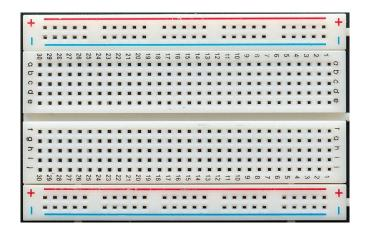
The breadboard is used as the platform for where all the electrical components (ultrasonic sensor, LED's, motor) are connected. From here, the inputs and outputs of the components can be connected to the Arduino.
