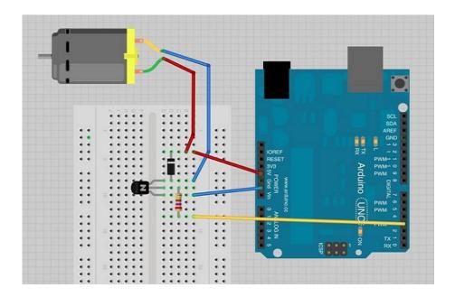
**NOTE:** The diagram should above uses an NPN transistor, although we are using a PNP transistor. To accommodate for this, switch the collector and emitter pins of the transistor. This can be done by simply placing the transistor to opposite way (flat face facing away rather than facing toward you).
